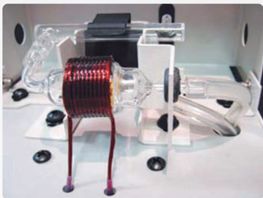
The RF coil surrounds the mercury concentration cell shown in front of the absorption cell located in the light path.
